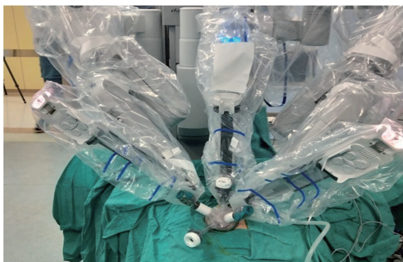
图 3 单孔 PORT 与机器人相连 Figure 3 Single site port connected to robot
