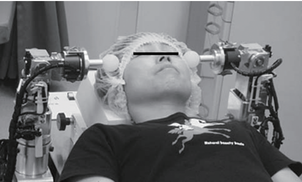
图 15 使用口腔康复机器人 WOA-1 对志愿者进行按摩 [49] Figure 15 Volunteers were massaged with the oral rehabilitation robot WOA-1
